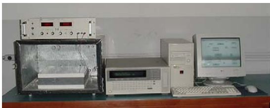
Figure 3 – Experimental apparatus used for determining \alpha and \lambda
